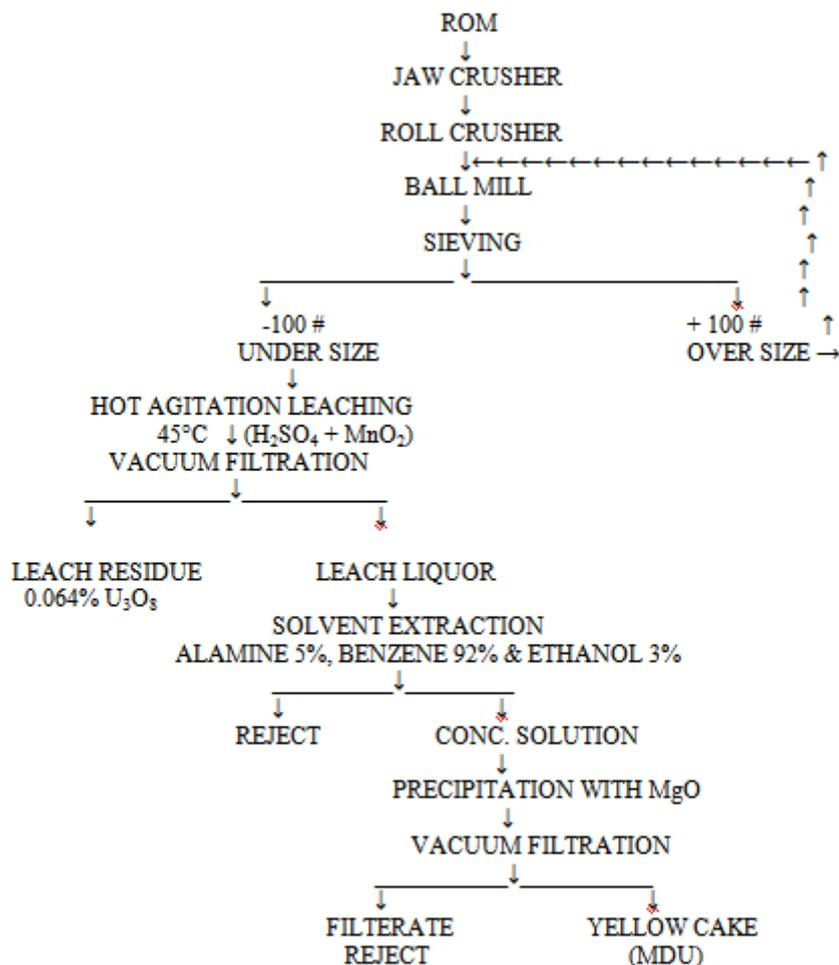
Fig. 8. Flow-Sheet for mineral processing of the Uranium ore (Sericite-chlorite-quartz-hematite phyllonite) from the Mulapalle area, Andhra Pradesh, India.
